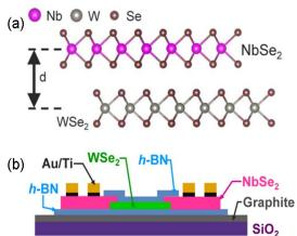
FIG.1. WSe<sub>2</sub> field-effect transistor with conducting NbSe<sub>2</sub> leads in side view. Atomic-model representation of the NbSe<sub>2</sub>/WSe<sub>2</sub> interface (top) and schematic structure of the device (bottom). (From Ref. [2]).
