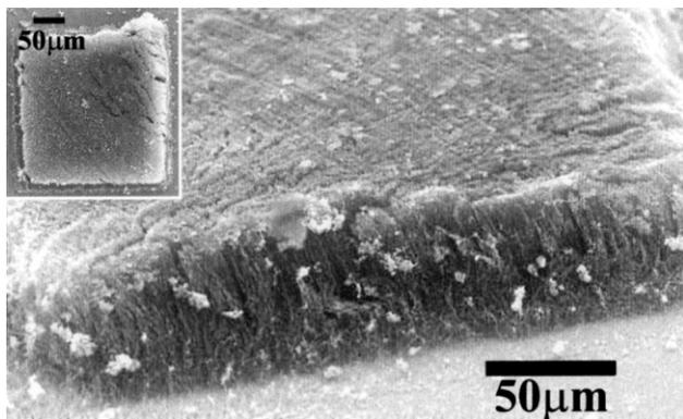
Fig. 3. SEM micrographs show the patterned nanotubes ( $250 \times 250 \mu\text{m}^2$ ).
