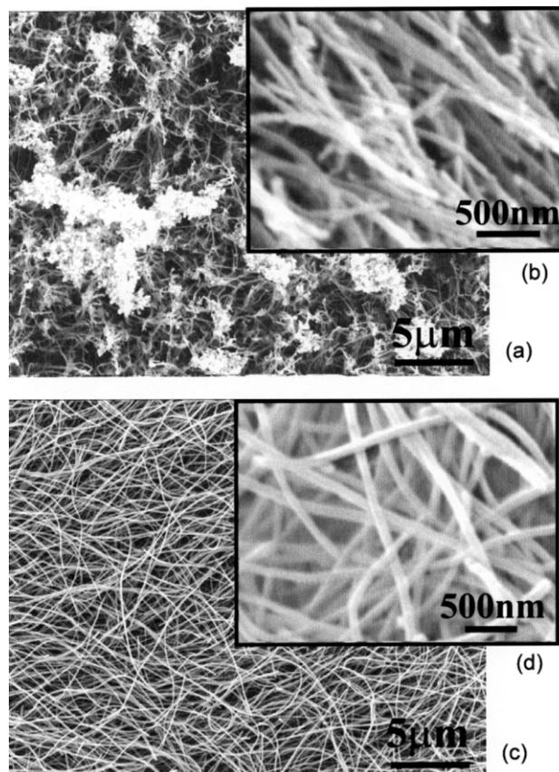
Fig. 4. SEM images of as-grown nanotube films (a and b) and films that have been subjected to ultrasonic treatment in methanol (c and d), resulting in removal of carbon clusters.
