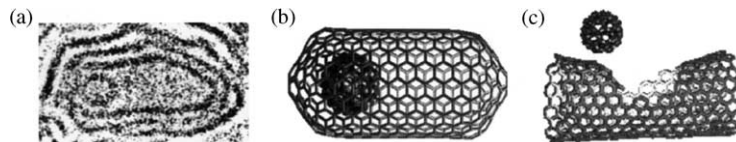
Fig. 3. (a) Transmission electron microscope image depicting a multi-wall carbon nanocapsule. This simplest “peapod” with a single C_{60} molecule was formed by thermal annealing of nanodiamond powder. (b) The structural counterpart, a C_{60}@C_{480} bucky shuttle. (c) A possible scenario of the peapod formation, involving a large vacancy in the tube wall. (a) and (b) are reproduced from Ref. [5] (© American Physical Society 1999).
