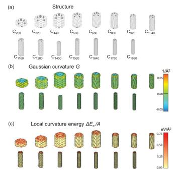
FIG. 8. (Color online) (a) Structural models, (b) local Gaussian curvature G, and (c) local curvature energy  $\Delta E_c/A$  across the surface of torus isomers with different heights H, defined in Fig. 6(a). The nonhexagonal rings in (a) are shaded. The values of G and  $\Delta E_c/A$  have been interpolated from their values at the atomic sites.
