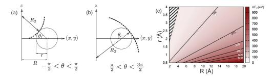
FIG. 3. (Color online) Definition of the principal radius  $R_2$  of a nanotorus in (a) its interior and (b) its exterior part as a function of the zenith angle  $\theta$ . (c) Contour plot displaying the out-of-plane curvature energy  $\Delta E_c(R,r)$  of nanotori according to Eq. (11).
