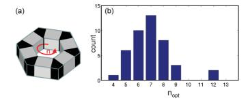
FIG. 10. (Color online) (a) A schematic model of a polygonal nanotorus with an n-fold (n = 6 in this case) symmetry. (b) Distribution of the optimal rotational symmetry numbers  $n_{\rm opt}$  in the 43 families of polygonal nanotori covered in this study.
