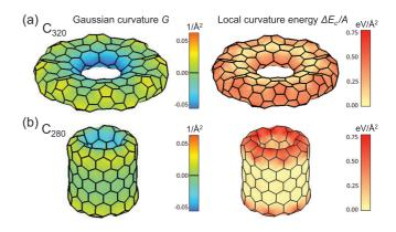
FIG. 5. (Color online) Local Gaussian curvature G(left panels) and local curvature energy  $\Delta E_c/A$  (right panels) across the surface of selected nanotori. Representative examples shown are (a) the flattened  $C_{320}$  nanotorus with 320 atoms and (b) the elongated  $C_{280}$  nanotorus with 280 atoms. G and  $\Delta E_c/A$  are interpolated from their values at the atomic sites.
