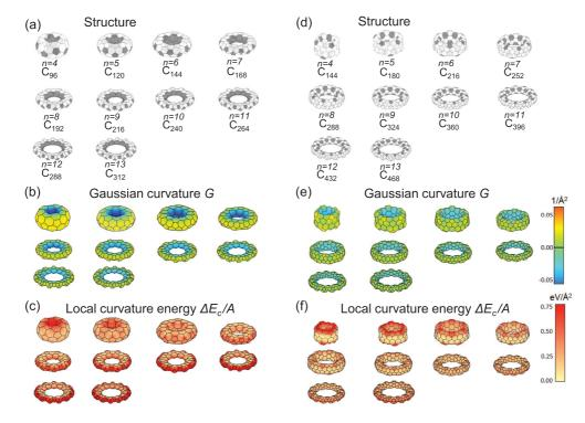
FIG. 9. (Color online) [(a) and (d)] Structural models, [(b) and (e)] local Gaussian curvature G, and [(c) and (f)] local curvature energy  $\Delta E_c/A$  across the surface of torus isomers with different rotational symmetry numbers n, defined in Fig. 6(a). Structures in [(a) and (c)] and [(d) and (f)] represent two distinct torus families. The nonhexagonal rings in (a) and (d) are shaded. The values of G and  $\Delta E_c/A$  have been interpolated from their values at the atomic sites.
