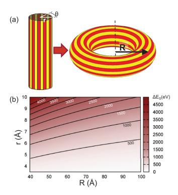
FIG. 2. (Color online) (a) Schematic of a striped nanotube (left), which is bent to a nanotorus (right). (b) Contour plot representing the in-plane strain energy  $\Delta E_s(R,r)$  according to Eq. (9).
