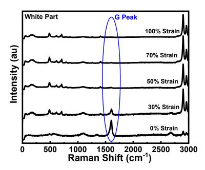
**Figure S5.** In situ Raman Spectra of the SWCNT@PDMS (white part) at particular strains during initial strain cycle  $(0\rightarrow 100\%)$ ).
