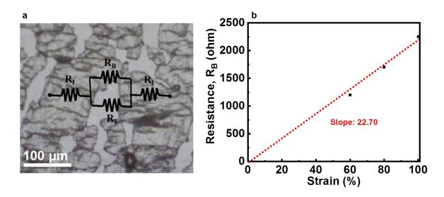
**Figure S8.** Resistance model (a) to describe the mechanism in resonse to applied strain and (b) Linear variation of R<sub>B</sub>, bridge resistance with applied strain (higher strain).
