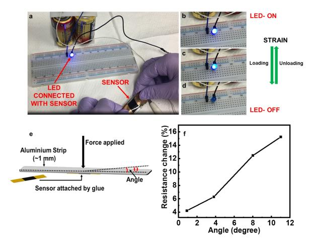
**Figure S12.** Real time response of the sensor in electrical circuit connected to LED (a), under applied strain (b-d). Loading of strain decreases the illumination intensity of LED whereas unloading of strain follows the opposite trend. (e) Schematic showing attachment of sensor to aluminium strip and (f) Resistance change with applied strain (change in angle) to monitor the structural integrity of aluminium strip.
