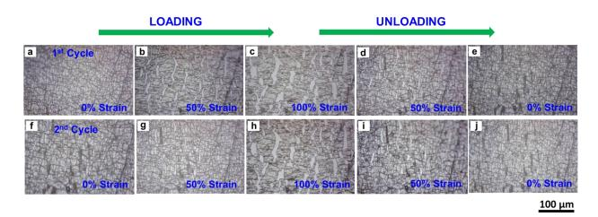
Figure S4. Optical Micrographs of SWCNT@PDMS during first (a-e) and second (f-j) loading-unloading  $(0\% \rightarrow 100\% \rightarrow 0\%)$  cycle.
