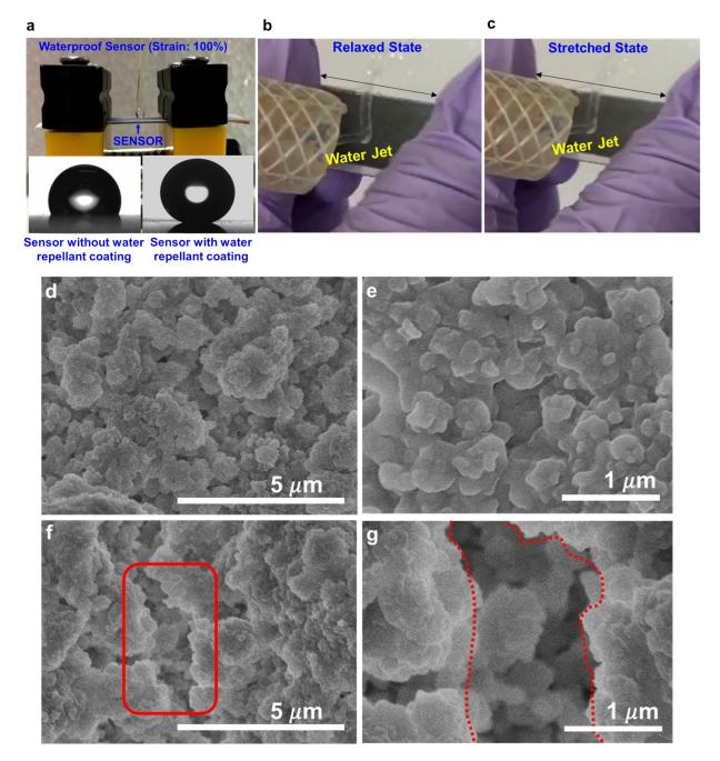
**Figure S2.** (a) Photographic image of waterproof sensor at 100% strain, inset shows water droplet on the surface of sensor with and without water repellant coating, Photographic image of water jet blocking at relaxed (b) and strained surface (c) of waterproof sensor, SEM micrographs of sensor under unstrained (d and e) and strained (f and g) states.
