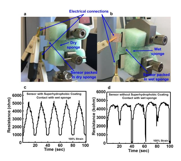
**Figure S3** Image of the water proof sensor packed in sponge under dry (a) and wet (b) conditions, Actual response of the sensor in contact with wet sponge (c) with and (d) without superhydrophobic coating.
