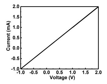
Figure S6. Current (I) - Voltage (V) Characteristics of Embedded Strain Sensor (PDMS/SWCNT/PDMS).
