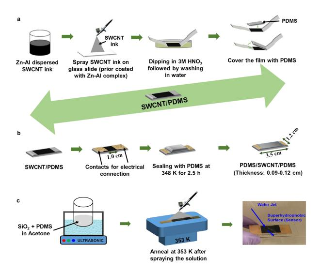
**Figure S1.** (a) SWCNT film formation process and transfer of film onto PDMS (SWCNT/PDMS), (b) Fabrication of embedded sensor, (PDMS/SWCNT/PDMS) and (c) Encapsulation of the fabricated sensor in water repellant coating (blue arrow shows the direction of water jet).
