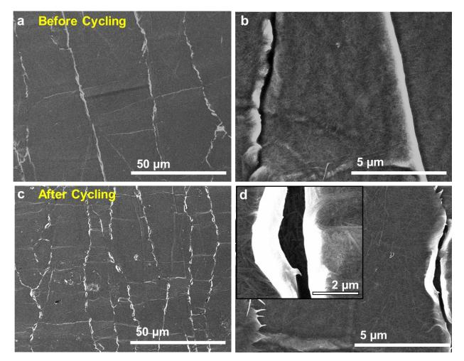
**Figure S11.** SEM micrographs of embedded sensor (PDMS/SWCNT/PDMS) before (a,b) and after 15k loading-unloading cycling (c,d).
