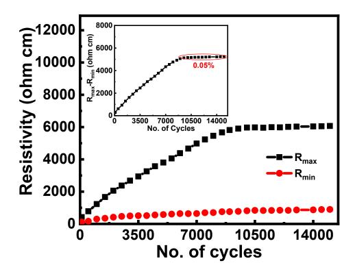
Figure S9. Change in resistivity of the sensor during 15k loading-unloading cycles.
