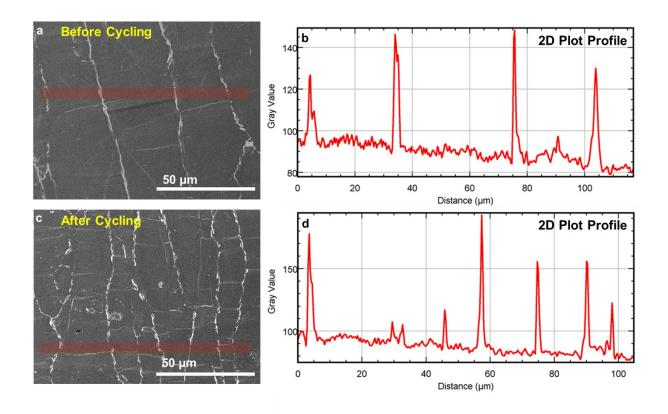
**Figure S10.** Analysis of SEM micrograph for 2D Profile by Image J software of the sensor, before (a,b) and after 15k cycling (c,d).
